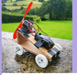
'I learned how to put a motor in a circuit and how to change the way it spins.
