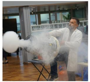
When the pressure increases above the pressure outside the container, the air inside the container is forced out through the hole. This is where it gets interesting.
